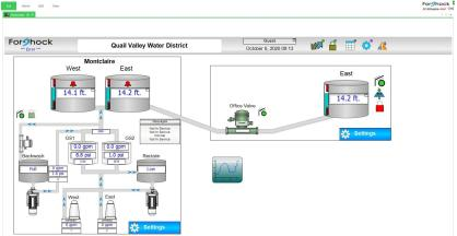
roschock\* display water tank levels, east tank valve operation and treatment plant pump operation. Programming is ongoing to add well status information and other data.
